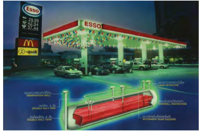
Esso uses double wall underground tanks at our service stations to minimize risk to the environment.
