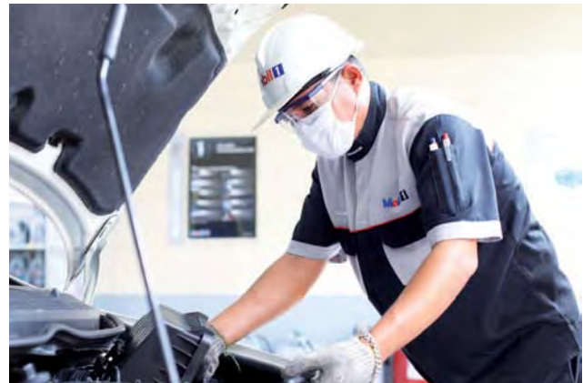
A Mobil 1 Center mechanic is changing an air filter after completing motor oil change for a customer.
