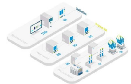
Picture depicts the structure of substation control and protection system according to IEC61850 standard
