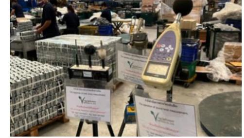
Inspection working environment (Sound measurement)
