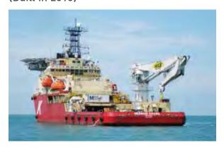
The DSV 'Mermaid Asiana' is a purpose-built DP2 dive support and light construction vessel. The vessel is equipped with a built in 12-man single bell saturation diving system complete with a self-propelled hyperbaric lifeboat. The vessel also has a 100-tonne active heave-compensated knuckle boom crane and accommodation for 100 personnel. This vessel is designed for operations in the Middle East and Asia-Pacific region. The DSV 'Mermaid Asiana' is ABS classed and flies the Panama flag.
