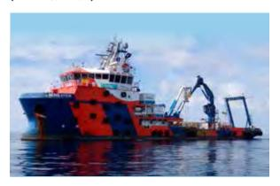
The RSV 'Resolution' is a DP2 ROV and diving support vessel chartered-in by Mermaid's Indonesian unit. The vessel has been specially modified for IRM duties and construction support tasks and is also capable of geophysical and geotechnical survey. This vessel is equipped with a 20-tonne main crane, 3-tonne general purpose crane, 25-tonne A-frame and accommodation for 60 personnel. The RSV 'Resolution' is Bureau Veritas/ BKI classed and flies the Indonesia flag.
