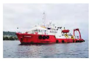
The SS 'Barakuda' (formerly MV 'Mermaid Supporter') is a utility vessel equipped with an omni-directional bow thruster and accommodation for 30 personnel. This vessel has an extensive track record for performance of platform inspection and FPSO (Floating Production Storage and Offloading) facility underwater inspection projects in South-East Asia using a combination of ROV and surface diving methods. The SS 'Barakuda' is DNV classed and flies the Indonesian flag.
