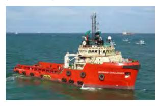
The MV 'Mermaid Challenger' is a DP1 offshore support vessel with 72-tonne bollard-pull capacity, and is also suitable for performing ROV support vessel duties. This vessel can be equipped with heavy work-class ROVs and has accommodation for 38 personnel. Originally built as an anchor handling and tug supply vessel, the vessel has supported offshore operations in Vietnam for the past few years. The MV 'Mermaid Challenger' is DNV classed and flies the Panama flag.
