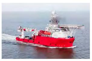
The DSV 'Windermere' is a purpose-built DP2 diving support vessel. The vessel is chartered-in by Mermaid's Indonesian unit and has worldwide capabilities. The vessel is equipped with a built in 15-man saturation diving system complete with a self-propelled hyperbaric lifeboat. The vessel has a 50-tonne active heave-compensated subsea crane, a 40 tonne active heave-compensated crane and accommodation for 120 personnel. The DSV 'Windermere' is ABS classed and flies the Indonesian flag.
