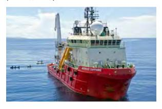
The RSV 'Mermaid Sapphire' is a DP2 remotely operated vehicle ("ROV") support vessel equipped with a deepwater work-class ROV, a 23-tonne knuckle boom crane and accommodation for 60 personnel. In 2012, the vessel supported James Cameron in his historical deep sea dive to the Challenger Deep, the world's deepest point in the Pacific Ocean's Mariana Trench, 10.99km below ocean surface. The RSV 'Mermaid Sapphire' is ABS classed and flies the Panama flag.
