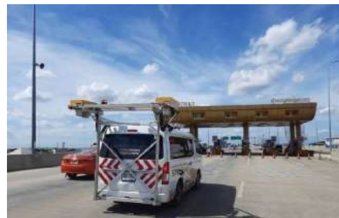
Pavement inspection: IRI and Rutting measurements
