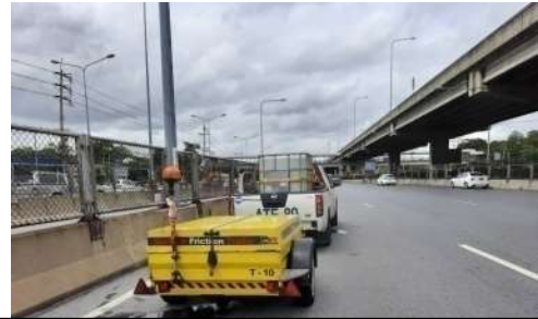
International Friction Index (IFI) Skid Resistance Tester using Fixed Slip Method
