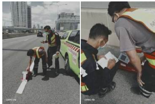
Inspection of lane marking reflectivity
